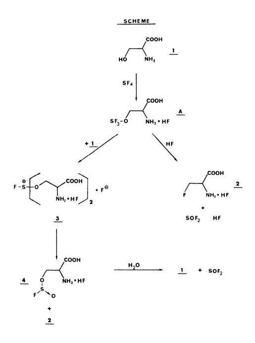
Racemic serine results support 3. When the two serines in 3 are both R- or both Sthe tetrahedral sulfur is achiral; the single  $^{19}$ F resonance at -19.0 ppm appears. With R,Sor S,R- combinations, sulfur becomes chiral and two diastereotopic resonances at -18.0 and -20.3 are seen. The statistical 1:2:1 pattern we observed with racemic serine is consistent with structure 3.<sup>5</sup>
